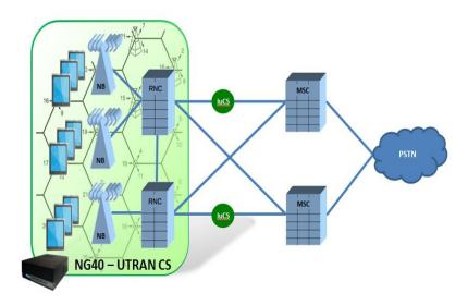
SW Bundle: RAN side DEMONSTRATION TEST emulator for multiple RNCs and NodeBs with Control Plane and User Plane functionality over Ethernet
