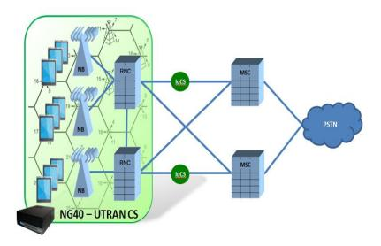
SW Bundle: RAN side FUNCTIONAL TEST emulator for multiple RNCs and NodeB with ControlPlane and UserPlane functionality over Ethernet
